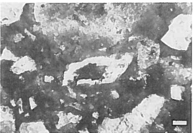
Figure 15. Plagioclase grain in poorly sorted sandstone with clay matrix. The center of the plagioclase grain has dissolved and the resulting pore is filled with oil. Scale bar equals 0.01 mm.
